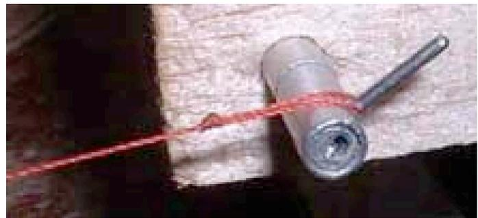
I found that a thin 2.5in. rubber band stretched to 5in. when you hook the line (braided cotton) on to the timer, right, provides enough pull for a positive release which is, of course, essential. My workshop experiment, at 60deg F worked out like this:
