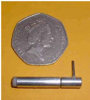
Assembly: Cyano the bearings in place on the shaft. Fix the sealing collar into the casing. Slide the shaft into the casing. Tamp in silly putty around the paddle and insert the end plug. Don't glue it in until you are sure that everything is running smoothly.
