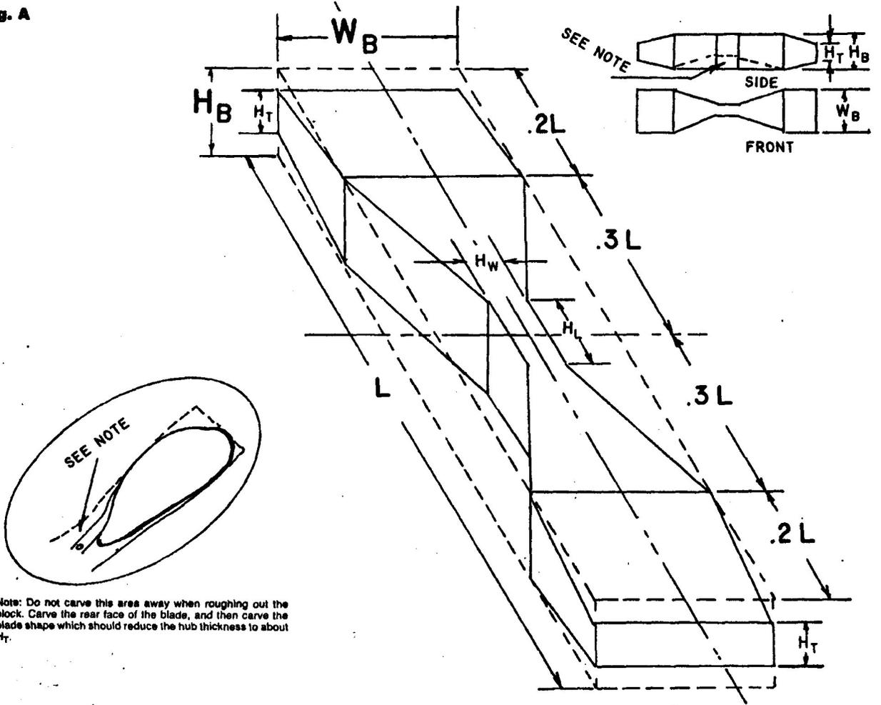
Note: Do not carve this area away when roughing out the block. Carve the rear face of the blade, and then carve the blade shape which should reduce the hub thickness to about  $H_T$ .
