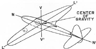
Grant defines stability as the capacity of an airplane to overcome any tendency to displace or turn from normal flight — or to return to normal flight after displacement.
