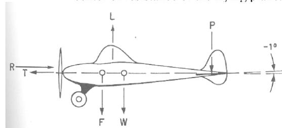
**Displacement factor #1, position of c.g. relative to wing lift** is illustrated in the diagram above. If the c.g. is located at W, behind the center of lift, it will tend to pull the tail down and create a stall unless the stab is designed to carry part of the load. When a non-lifting tail is used the c.g. must be located ahead of the line of lift (F). Grant's rule in this instance is to locate the c.g. of 1/3 the chord back from the leading edge.
