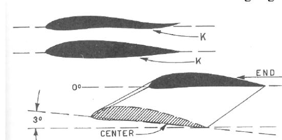
Grant offers three methods for reducing the shifting of the center of lift. The upturned trailing edge and the use of a symmetrical airfoil will accomplish the job. Neither airfoils are as efficient in terms of lift as a flat or undercambered airfoil, but the purpose here is to reduce center of lift shift. The third method is to sweepback the wing and wash out the angle of incidence toward the outer ends.
