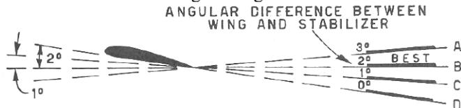
**Displacement factor #5, Speed.** If the stab is set at an angle less than the wing, given sufficient speed, it will tend to make the model climb or stall. It then may be asked why, if at considerable speed it tends to produce a deviation from level flight, should there be any difference. The reason is that this difference is important to recovery, so a slight difference must be maintained.
