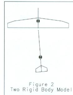
Now with the same centripetal formula we can calculate the force at the center of mass of the second body (the boom and Y-Tail). For our typical carbon boom and a 17" tail moment this is about 3 pounds. We can apply this 3 pound force to the tail boom and measure its deflection, about 2". Wow, that is a bunch! Now we can understand why TLGs need such strong joints.
