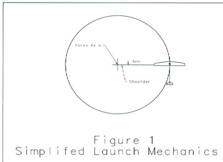
With this mathematical model we can calculate the centripetal force required to keep the model at this radius (How hard it is to hold a typical launch). The force is calculated by the formula:
