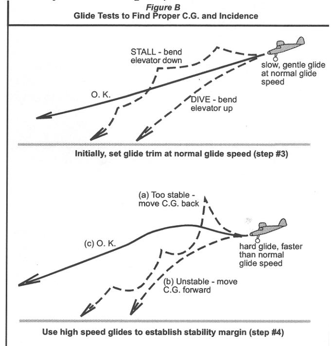
4. Continue gliding the model while slowly increasing the speed of launch, until you are tossing it considerably harder than a normal launch; about twice as fast at least. The shape of the model's trajectory at these higher speeds indicates how stable the model is.
